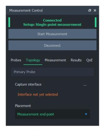
The Probe needs to know which network interface it is supposed to listen to during measurement. Select the interface by pressing ... on the right side of *Capture interface*. A dialog opens, which lists the interfaces of this computer.
