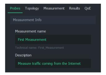
Next, define the measurement type. In a single-point measurement, only one Probe is used, yielding mainly traffic and flow statistics. In a two-point measurement, full QoS statistics can be measured in the network path between the selected Probes.
