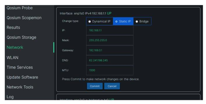
In addition to typical network settings, you can select interfaces to be bridged. By default, the two parallel network interfaces at the device's side are in the bridged mode. You can remove the bridging or change the interfaces in the bridge. You can bridge only two network interfaces at a time. Click *Commit* to save the changes.
