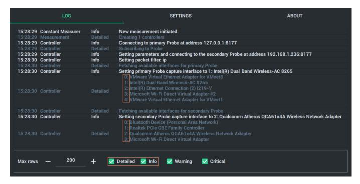
If, for example, we want to use Intel(R) Dual Band Wireless-AC 8265 (index 1) as the primary Probe capture interface and Qualcomm Atheros QCA61x4A Wireless Network Adapter (index 2) as the secondary capture interface, we would update the configuration file with the following information:
