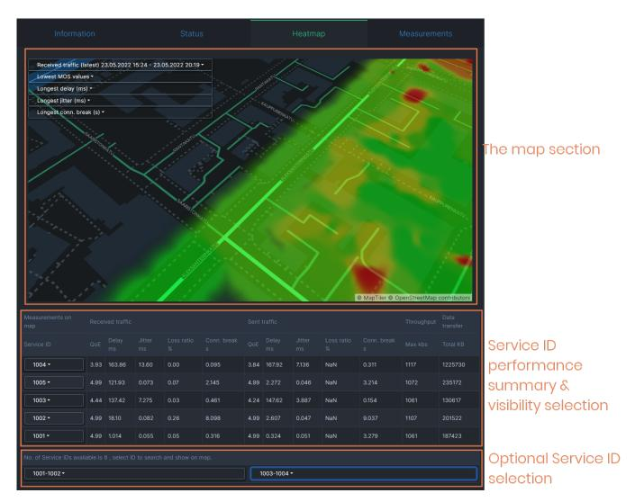
Qosium Storage's heatmap is currently tightly bound to Qosium Probes' **Service ID**. That is because **Service ID** is often used to distinguish devices in the field, making it a device ID. Thus, **Service ID** is the natural identifier according to which you can select results in the map. In addition to selection possibilities, the middle section in the Heatmap tab shows QoS summaries per **Service ID**.
