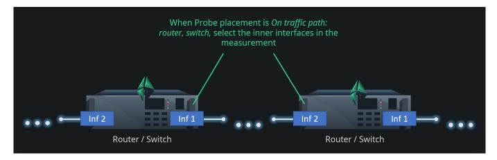
If the traffic or the network interfaces are such that there is no L2 addressing, you need to set the Sender parameters manually
