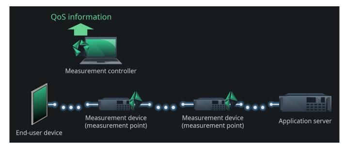
In this scenario, you need to pay some attention to the devices: how they operate and how they are connected. For example, a network bridge is considered as a passive device, and parameterized <u>accordingly</u>. The reason is that MAC addresses are used to define the flow directions in this mode, but it does not work for passive devices that just let the traffic through untouched like a network bridge does.
