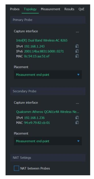
The new setting, NAT, is needed when there's a Network Address Translation between these two Probes. This is not the case in our setup, so we leave it unchecked.
