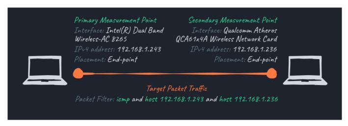
There can be—and most likely are—other packets traversing in and out of the involved interfaces than just our ping packets, and we want to exclude those from the measurement. This is where the *packet filter* comes into play.
